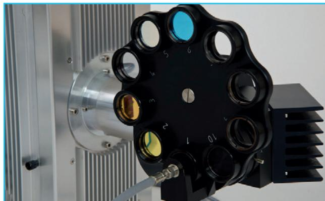
Manual filterwheel with 10 positions
