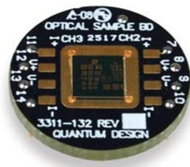
Figure 5: 1951 US Air Force Target mounted on a sample board and image of target taken using optical positioner software integrated into MultiVu.
