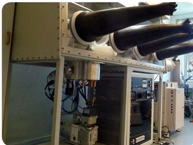
A modular MiniLab 026 system for installation into a glovebox
