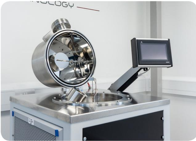
The MiniLab 026 with touchscreen HMI control and a 'clam-shell' type chamber, opened here to reveal internal techniques
