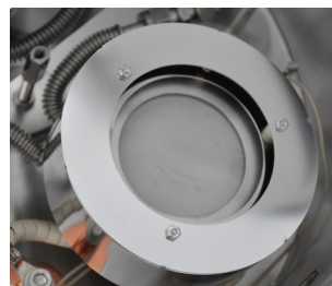
ABOVE: ANNEAL system LEFT: Quartz lamp stage with water-cooled enclosure and extra thermocouple CENTRE: Quartz lamp stage, platen removed RIGHT: SiC element stage for 1000 °C substrate temperatures
