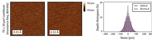
**Electrical Noise Level of 0.32 Å for Self-Sensing Cantilever equals Optical Noise Level**
