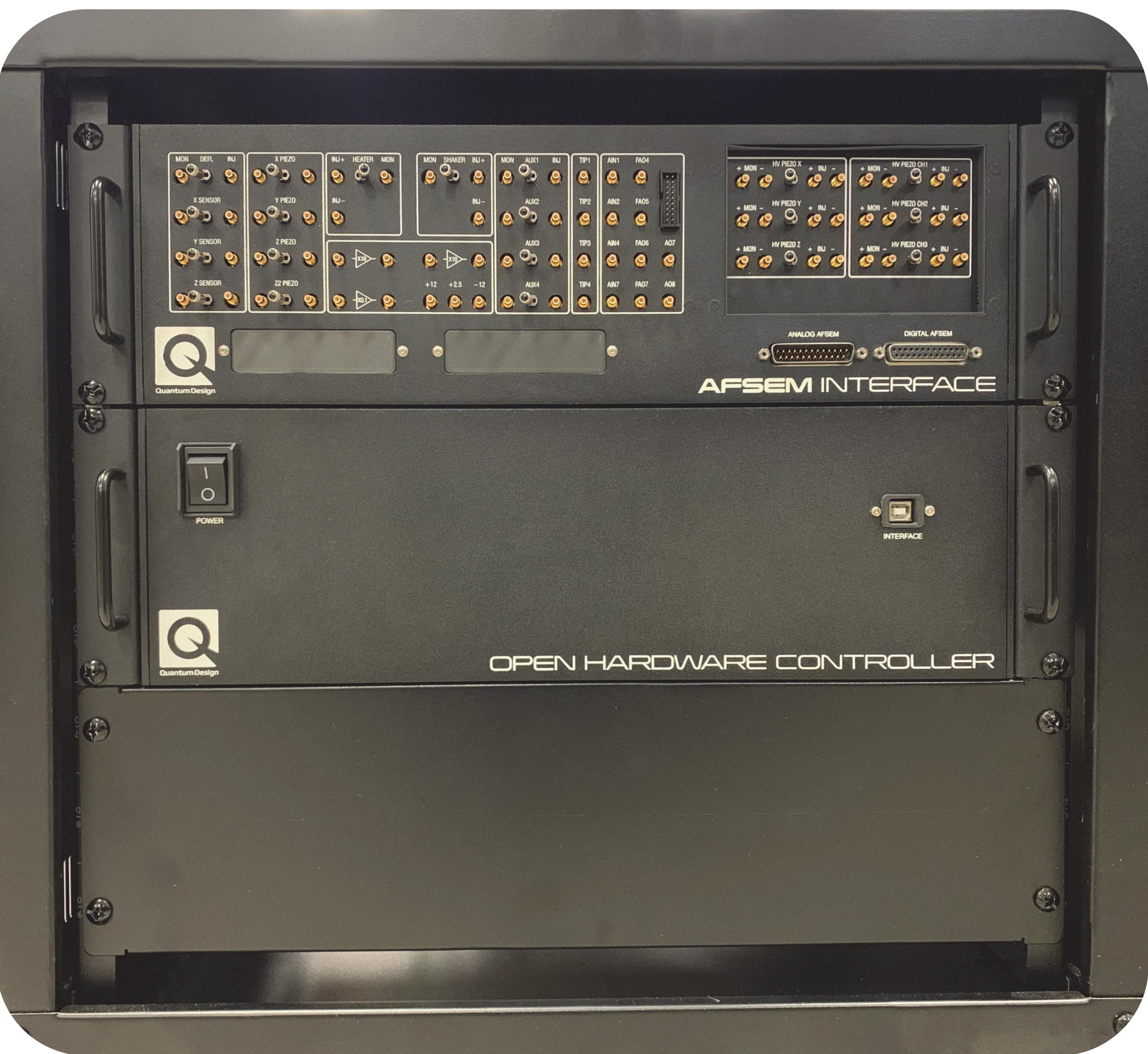
AFSEM controller consists of the Open Hardware Controller, a project started by EPFL, as well as the AFSEM Interface Unit. This controller opens a world of possibilities to implement novel ideas, thanks to auxiliary analog IOs and easy to program open-source LabView-based environment.
