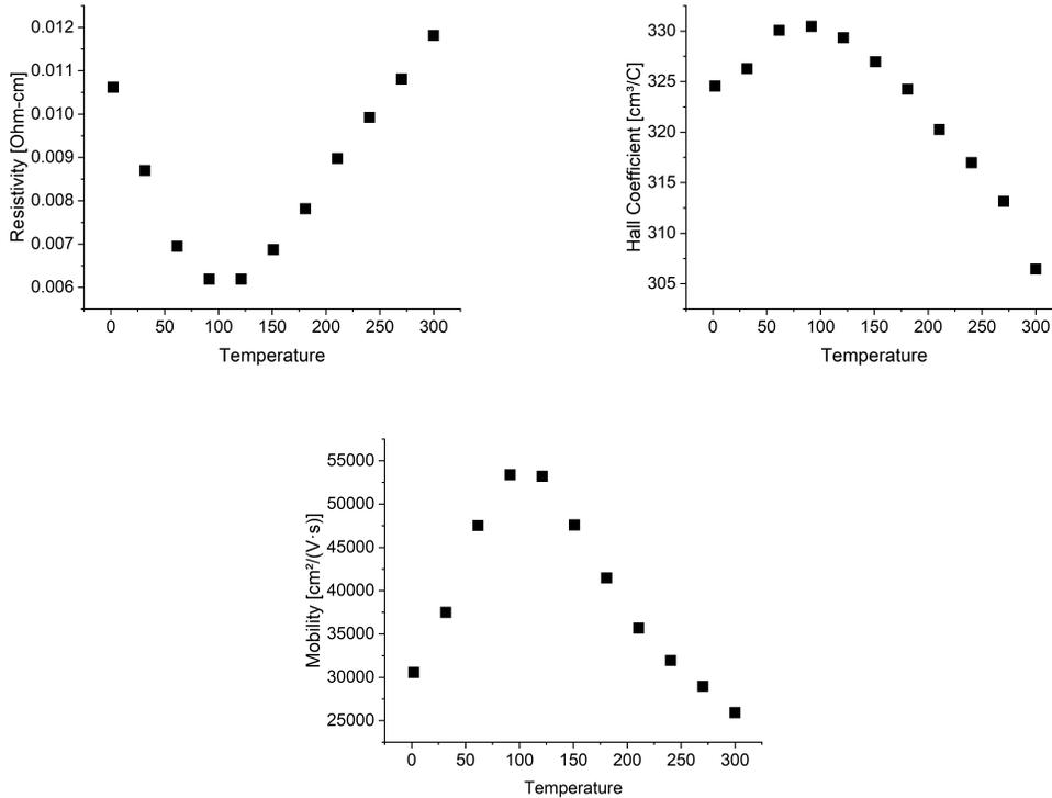
**Figure 5:** Resistivity, Hall coefficient, and mobility measurements of InAs from 2 K to 300 K measured in an OptiCool with the M91 FastHall measurement system.
