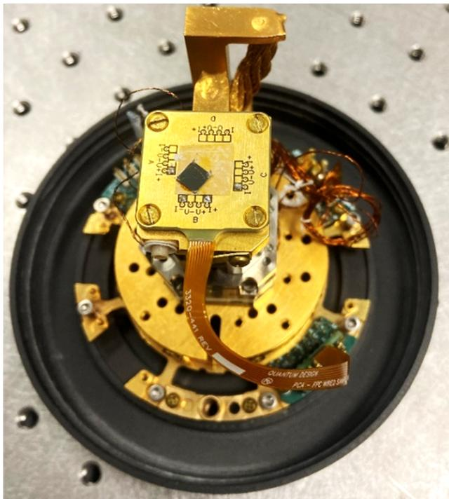
**Figure 4:** InAs sample mounted to Wired Sample Mount with insulating cigarette paper between the sample and sample mount.
