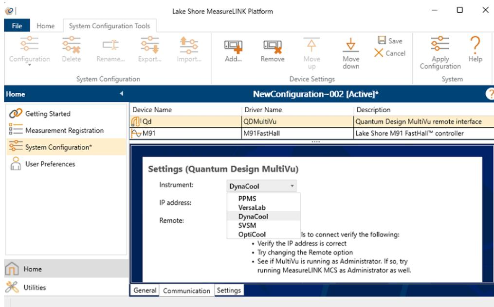
**Figure 2:** To setup MeasureLINK to use with the OptiCool, make sure the QD MultiVu Application package is installed and then under **Home > System Configuration > QDMultiVu > Communications**, select **OptiCool** from the **Instrument** dropdown.
