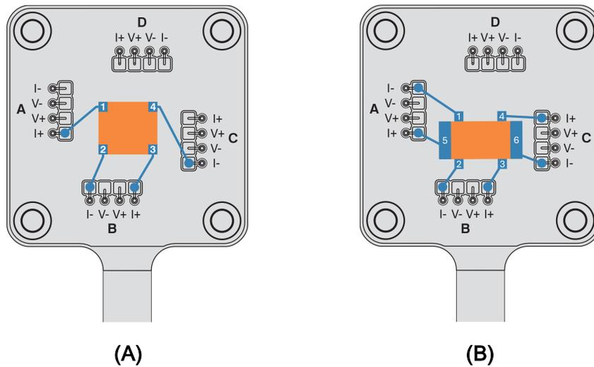
**Figure 3:** Wiring configurations for van der Pauw (A) and Hall bar (B) geometries on the Wired Sample Mount.
