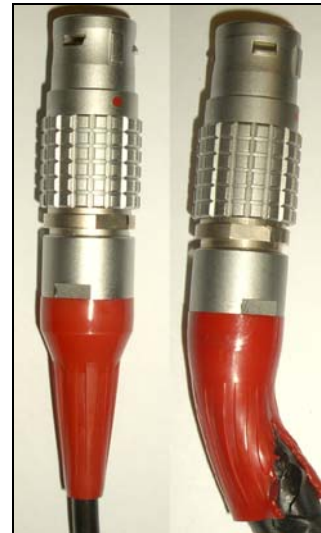
Figure 2. Comparison of Red Lemo cable before (left) and after (right) overheating.
