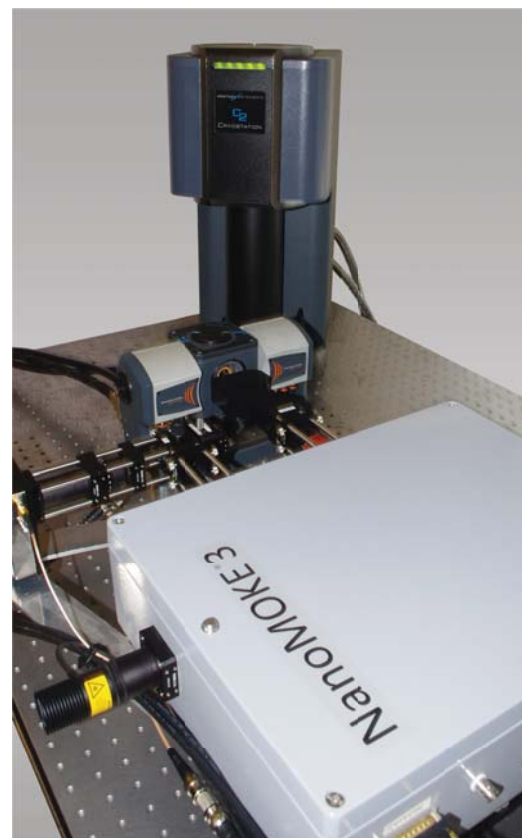
NanoMOKE® 3 incorporated into cryogen-free Montana Instruments Cryostation.
