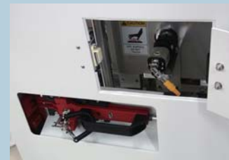
Focus adjust via front door
