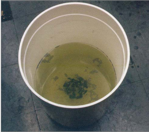
Demonstration of the removal of grinding swarf from machining fluid from a large-scale industrial facility using superconducting magnetic separation
