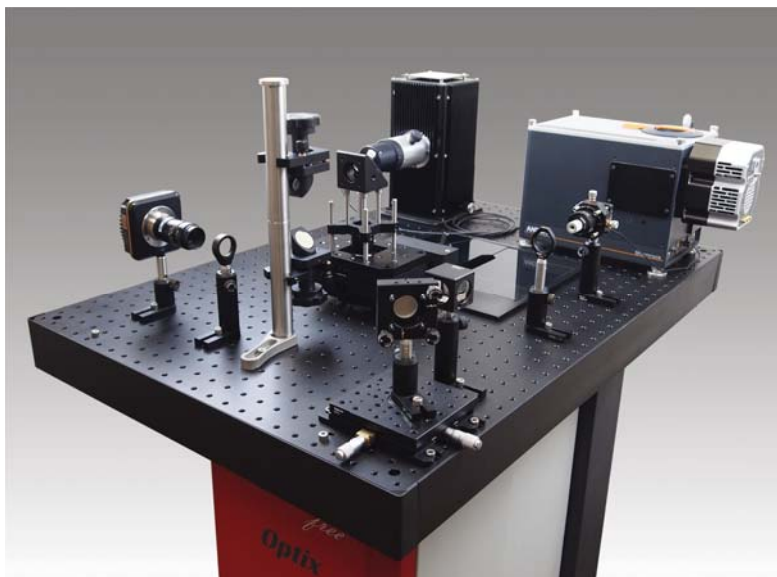
Figure 2: VersaLab Optix displaying its capability to set up external optical experiments in order to direct a laser beam down a VersaLab Optical Multi-Function Probe (OMFP).
