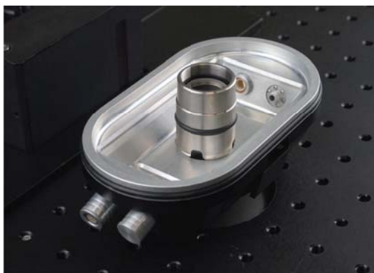
Figure 5: Optical Multi-Function Probe resting in the Wired Access Port on the Versalab Optix system. The Optical Wired Access Port has options for electrical or SMA Fiber optics connections to run wire or fiber optics to the sample.
