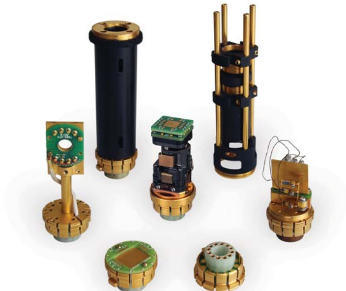
Figure 4: Optical and non-optical measurement option sample stages available for Versalab Optix.
