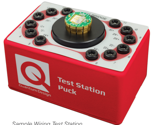
Sample Wiring Test Station
