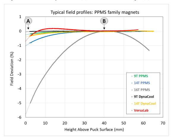
Because magnetometry measurements like VSM, torque and ACMS are most sensitive to magnetic field variations, they are positioned near the magnet center (B).
