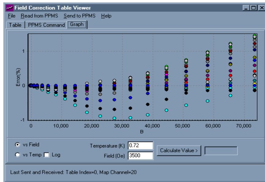
Figure 4: A typical calibration table plotted against Field
