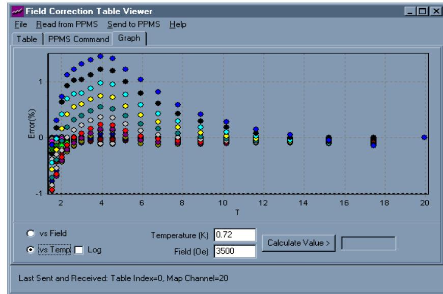
Figure 5: A typical calibration table plotted against Temperature
